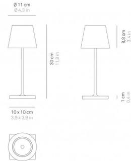
Poldina pro mini is a rechargeable table lamp, with contact charging base, painted aluminum body, polycarbonate diffuser and LED light source.
