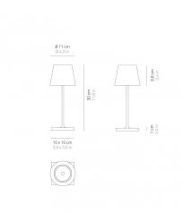
Poldina pro mini is a rechargeable table lamp, with contact charging base, painted aluminum body, polycarbonate diffuser and LED light source.
