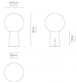
Olimpia pro is a battery-operated portable and rechargeable table lamp. It is equipped with: contact charging base, dimmer touch control and an amber accessory for changing the light colour (LED cover). It is not recommended to use the lamps with gold, chrome and silver finish for continuous outdoor use.
