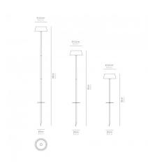
Sister Light lamp with peg is a battery-operated portable and rechargeable lamp. It is equipped with an electronic control system monitors the remaining autonomy and ensures constant luminous flux until the battery runs out. A customisable multifunctional touch control menu allows you to adjust the light colour temperature to 2700-3350-4000K (dynamic white) and to set or exclude the 4-step dimmer function.
